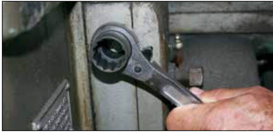
Ratchet podgers: For extra leverage on fasteners in confined spaces.
