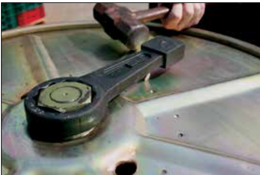
Sloggers: Ideal for loosening large nuts when extra force is required.
