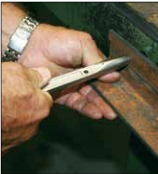
Ratchet podgers: Aligns bolt holes easily.
